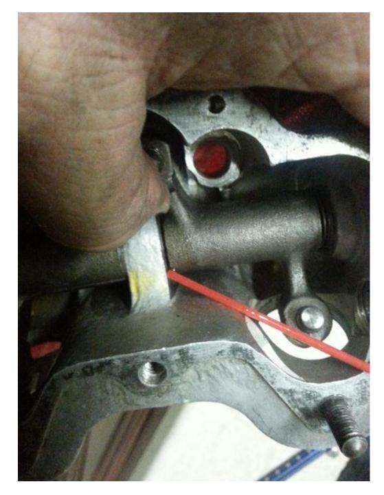
and then stuck an old pesola spring scale on them to see how much tension it would take to make the rockers of each type rock. i used to use the scale to weigh squirrels, but it works okay for rocker arms too:
