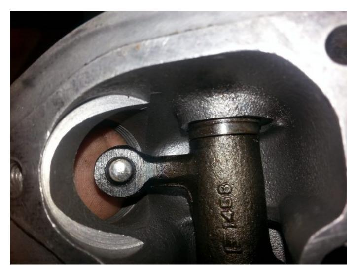
anyway, i lubed everything up as well as could through the hollow rocker shaft and from the outside with PB Blaster:
