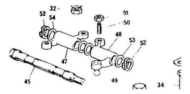
Note in the second illustration that part #54 (3/8") is labeled incorrectly and should read part #53 (1/2"). (Not to mention that the thrust washers are labeled backwards relative to the shaft orientation, but that's another can of worms!)
