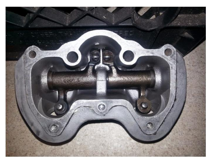
he installed the spacer against the rocker arm, in the same spot as the thackery washers in the other rocker box. these rockers don't have the little cutout:
