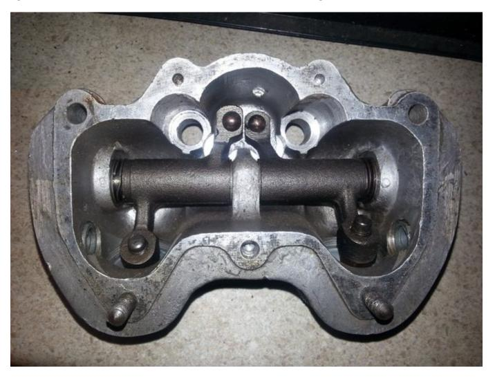
notice how the washer is digging into the oil cutout on the rocker arm:
